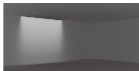
Wall Washer Lighting
